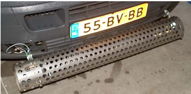
Ambient probe for vehicle mounted leak detection – shown with dust cover and cable shrouds removed
